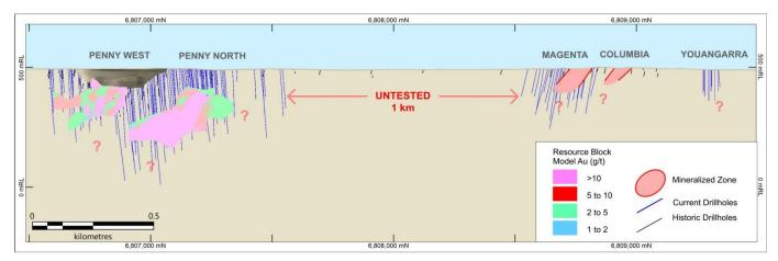
Figure 7. Long Section from Penny West past the Columbia Prospect looking West.
