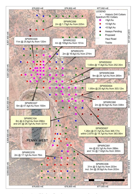
Figure 3. Drill hole collar plan at Penny North and Penny West
