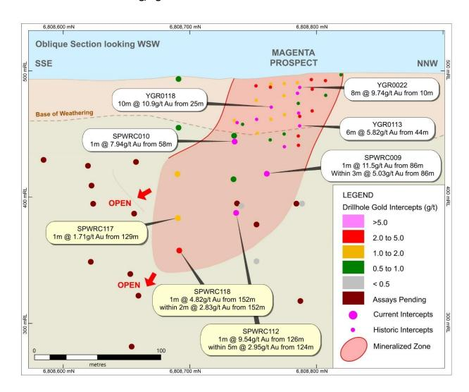
Figure 4. Long Section through the Magenta Prospect with significant intersections (refer ASX Announcement 30 April 2019 for previously reported information)
