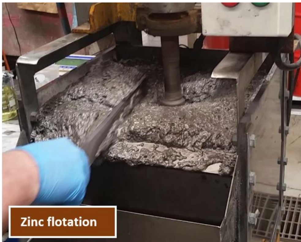
Figure 2. Zinc concentrate produced from zinc flotation test
