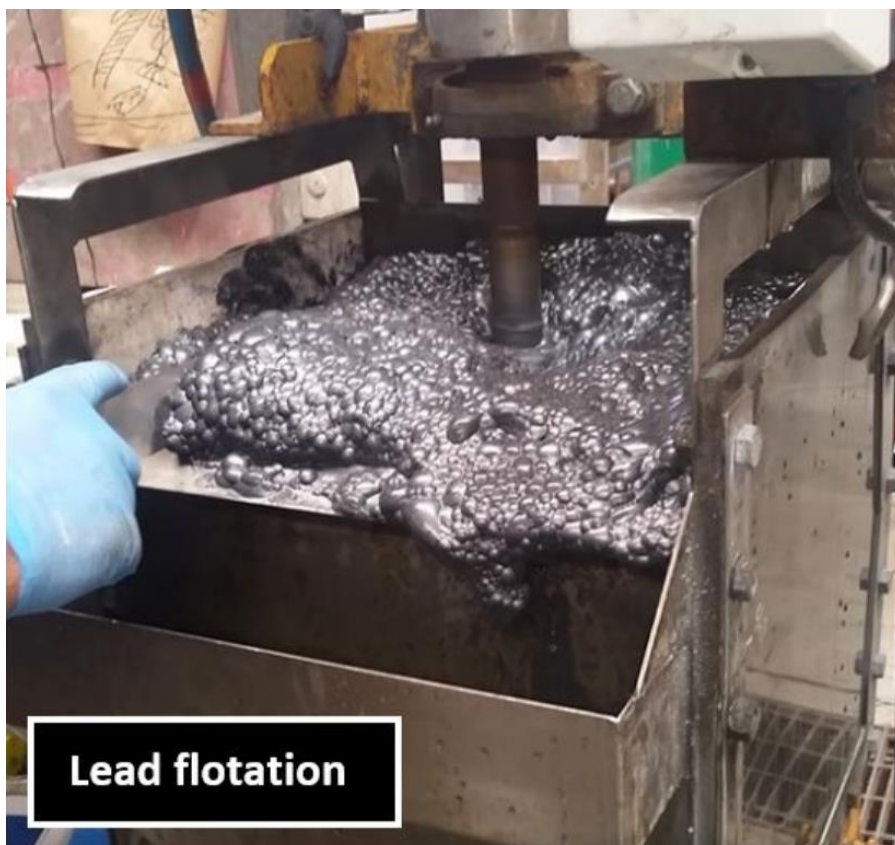
Figure 1. Lead -silver concentrate produced from lead flotation test
