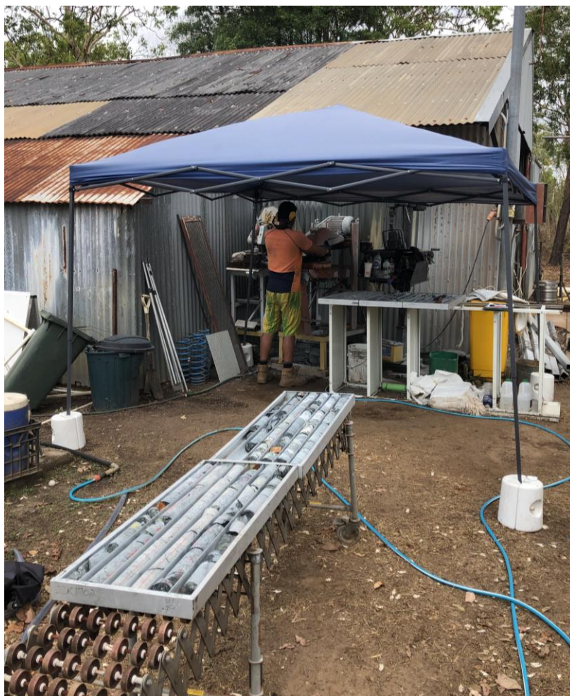
Processing of Diamond Drill Core Derived from Terrys Prospect
