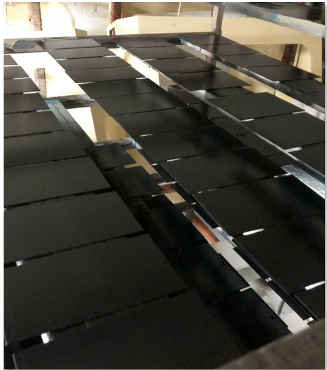
Figure 5 Spray coated test panels in drying chamber before going to Talga's corrosion control testing lab.
