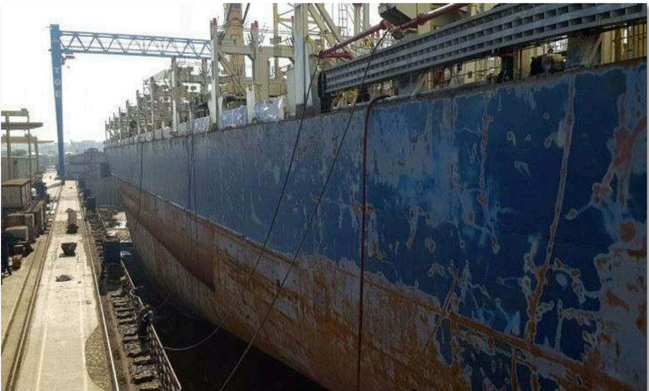
Figure 3 M/V Arica in dry dock with hull being stripped for repainting including Talcoat™-enhanced primer.
