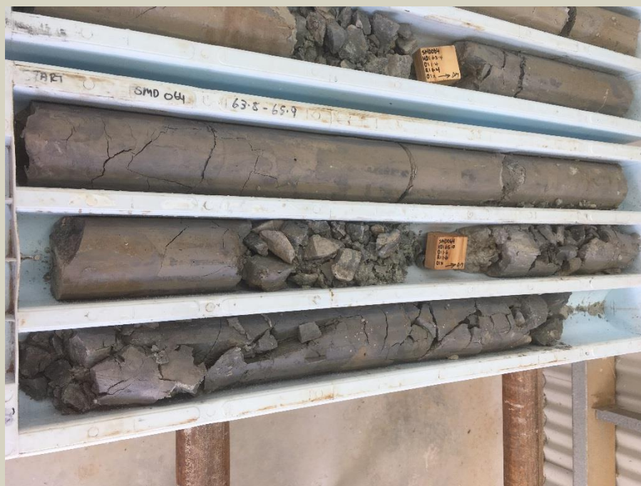
Clay altered sandstone at 63.0m.
