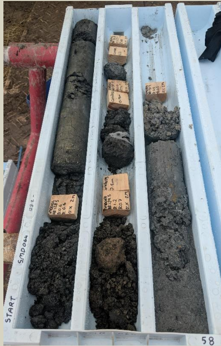
Core-loss zone at 129-130.8m.
