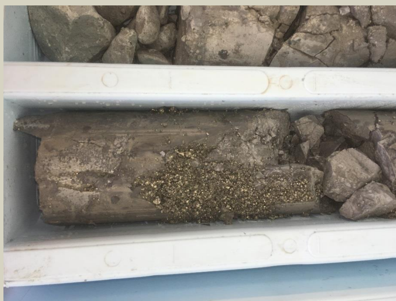
Massive Sulphide fracture fill in broken ground at 90.0m.
