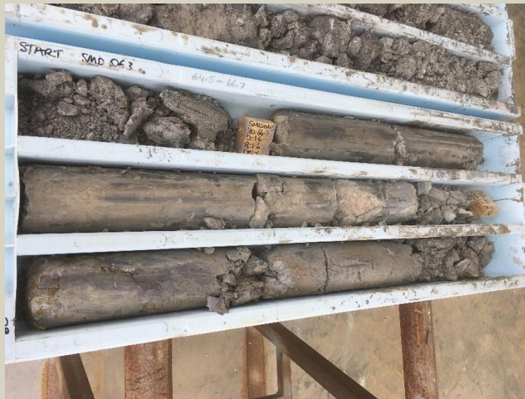
Clay altered sandstone at 64m.
