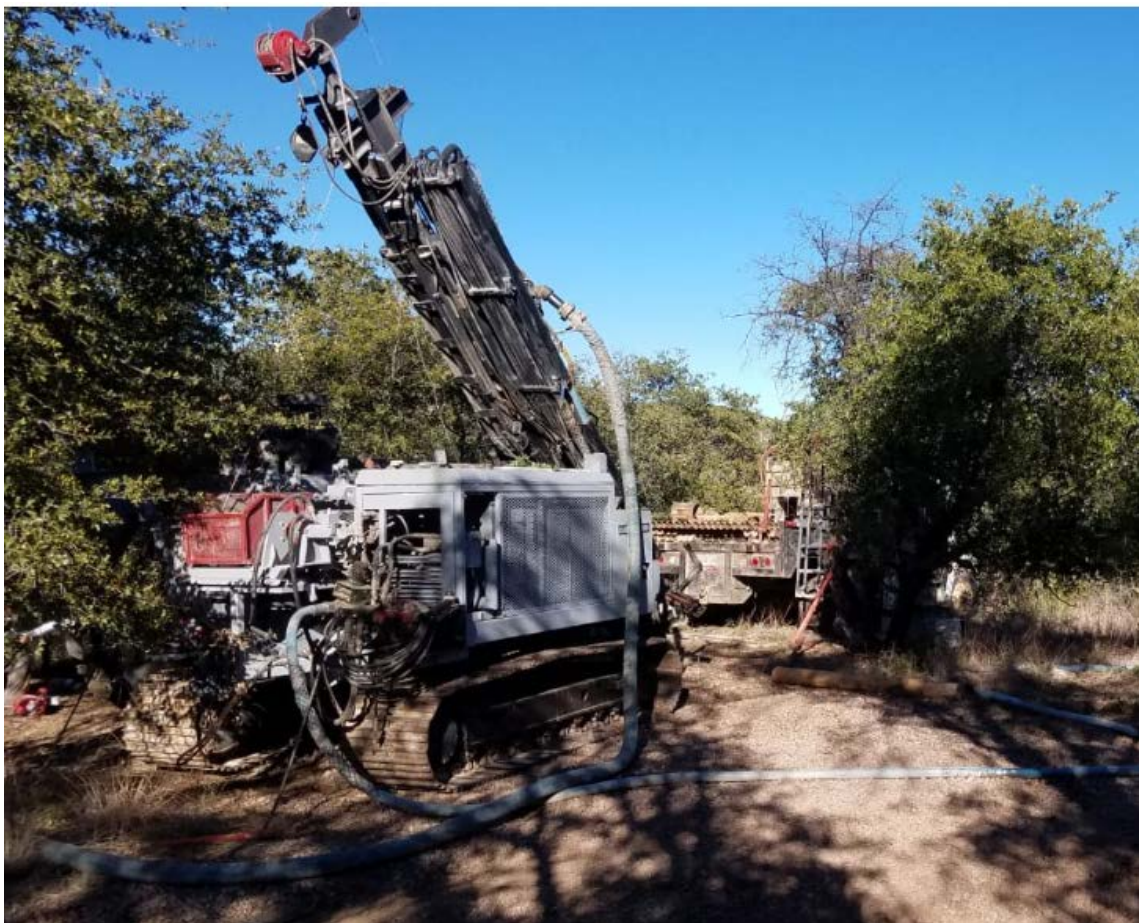
Photo 1: RC drill rig setting up at Loma Bonita
