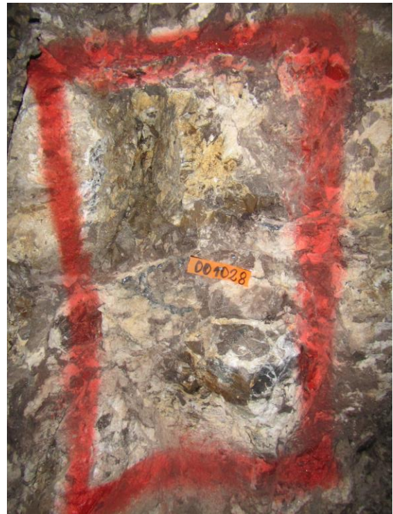
Figure 3 RIGHT : Typical ore at Cerro Rayas, exposed in drives at the Torrepatá mine working; dolomitised limestone (brown) brecciated with a calcite (cream) matrix. Galena, sphalerite and smithsonite occur in the breccia matrix and clasts.
