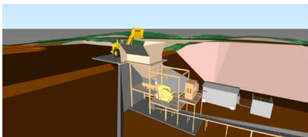
Figure 5: Crusher and surge bin
