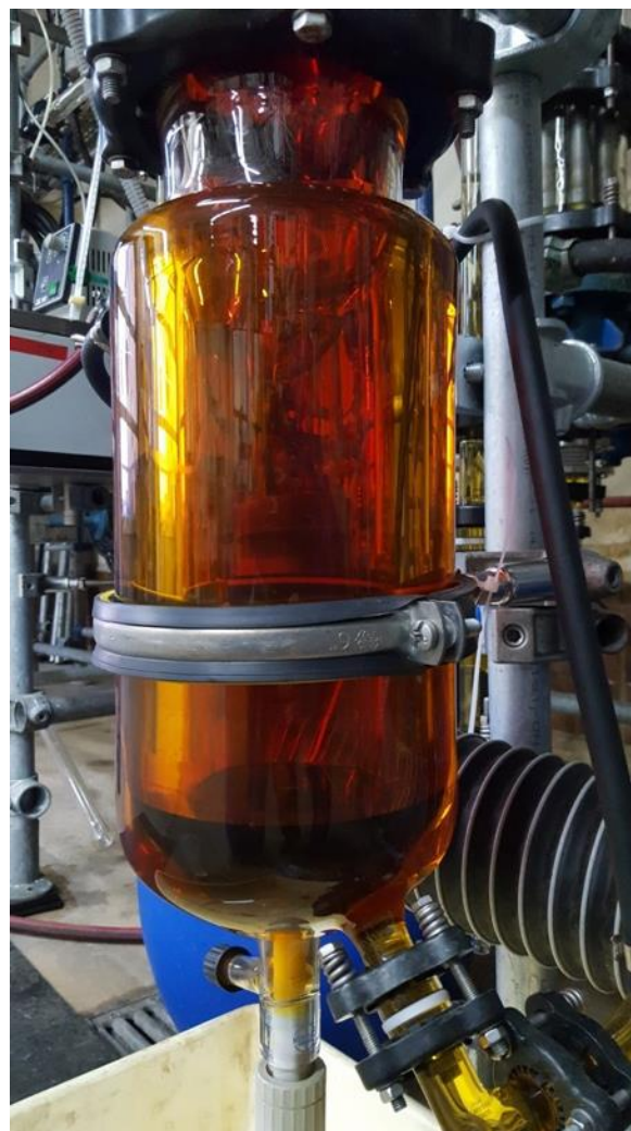
Figure 3: Reboiler with Bromine
