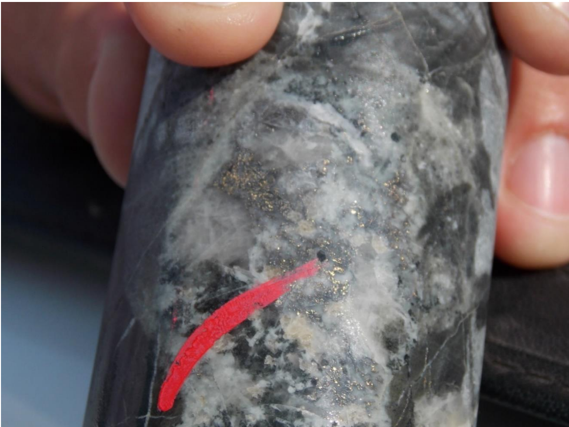
Figure 3: Photo of fine grained (sub-mm) disseminated visible gold and associated arsenopyrite intersected in MU19DD04 from 100.32m. Length of core shown is approximately 6cm.
