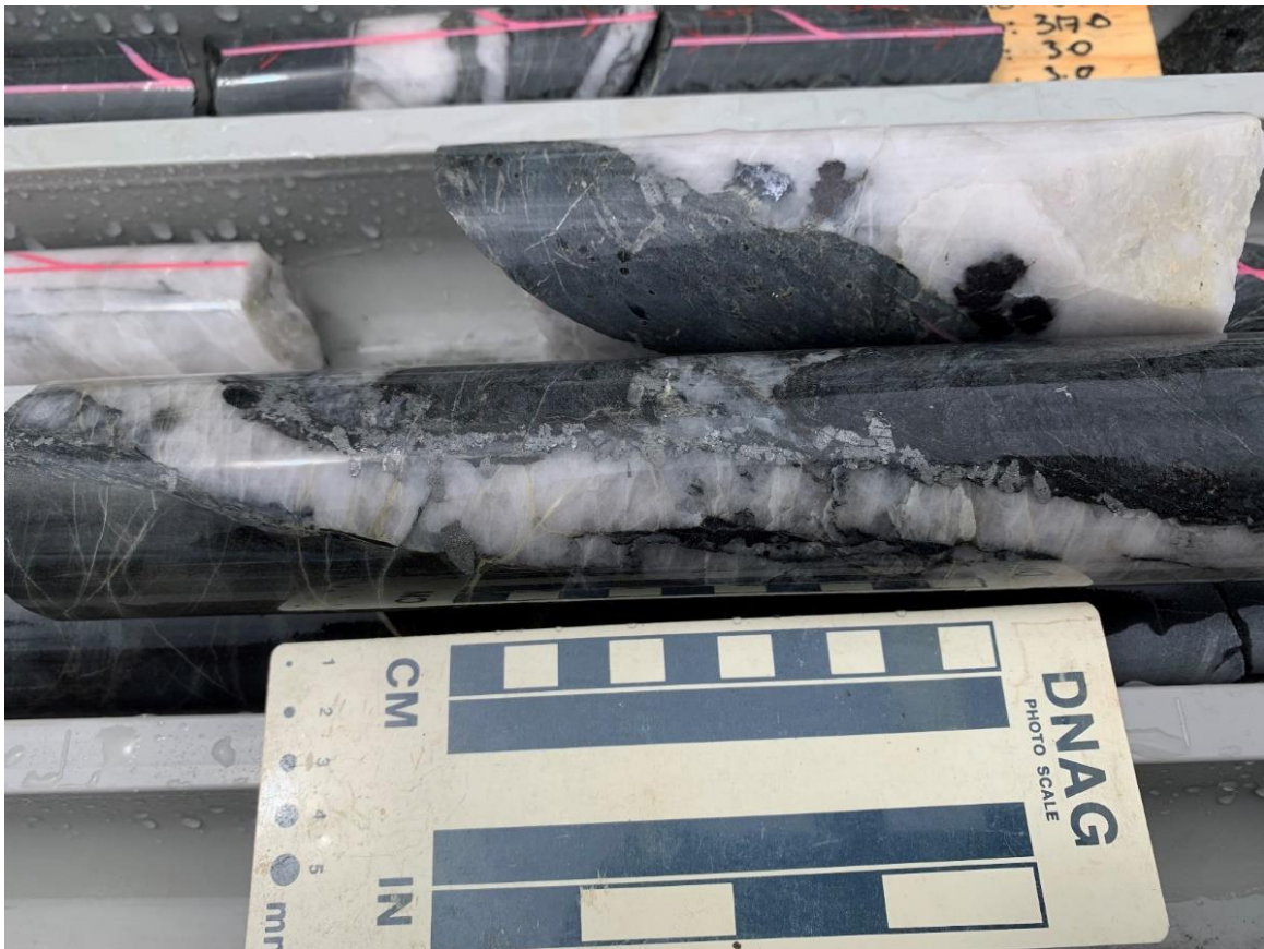
Figure 2: Close up photograph of mineralised quartz veins and sulphide alteration assemblages observed in MU19DD02 (at approximately 319.6m). Note coarse grained euhehedral arsenopyrite grains (foreground core sample) and coarse grained galena and sphalerite (background core sample) found near the margins of the quartz vein.
