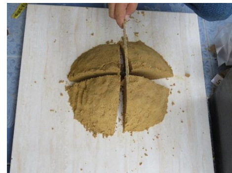
Figure 3-5 Cone and quartering of samples
