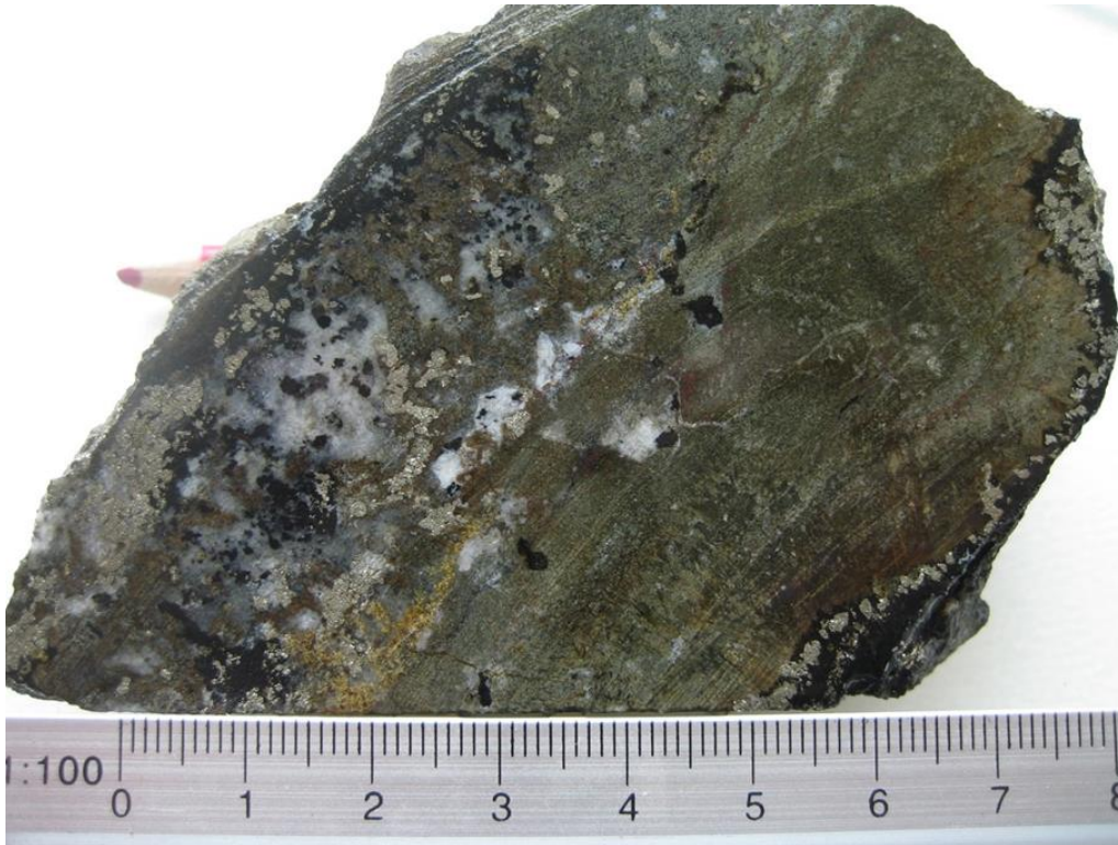
Photo 1 - Core from GNDD-003 - 59.45m (interval 59.0 – 60.0m assay: 65.6 g/t Au, 26.5 g/t Ag, 5.2 % Zn)
