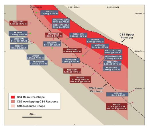
Figure 3: Zoom-in of Cassini long section depicting the CS5 Mineral Resource which partially overlays the CS4 Mineral Resource.
