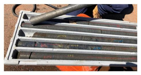
Figure 1: MDD339 core photo showing a section of heavy matrix nickel sulphides
