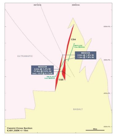
Figure 4: Cassini cross-section 6491350N with DHEM plates
