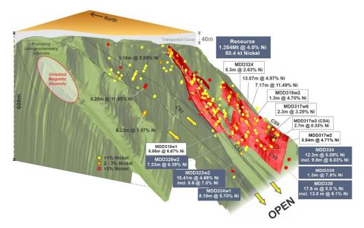
Figure 2: Cassini 3D image showing basalt surface and resource shapes with significant intersections
