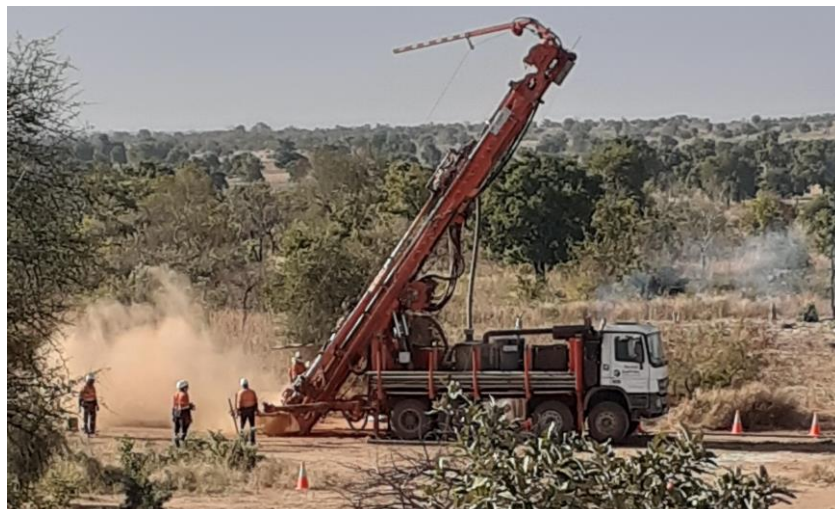
Figure 7: RC rig on site at Divole West on Hole DW-RC-19-001
