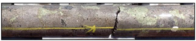
Massive pyrrhotite-chalcopyrite-pentlandite sulphide in drillhole RKDD007, 119m (NQ2 core)
