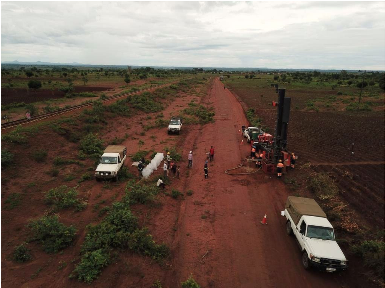
Figure 3. Air-core drilling at Railroad Prospect in December 2019.
