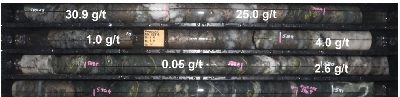
Figure 10: Northern STEP OUT diamond drill core from DRDD295, drill hole confirms high-grade mineralization associated with the DHEM plates to the north, 5% pyrrhotite, trace chalcopyrite and trace visible gold mineralization.
