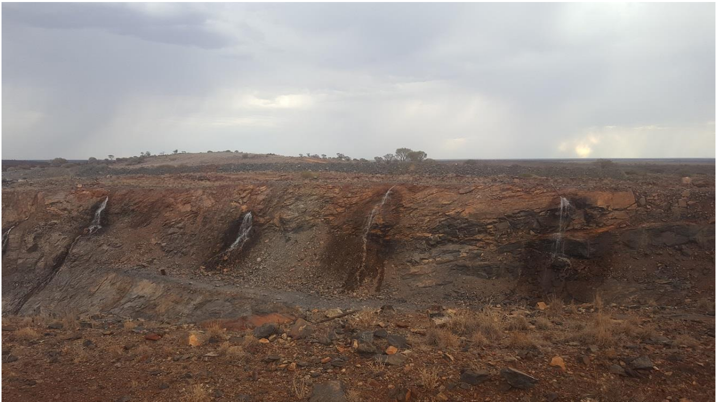
Figure 2: Water is being transferred from underground workings to existing open pits
