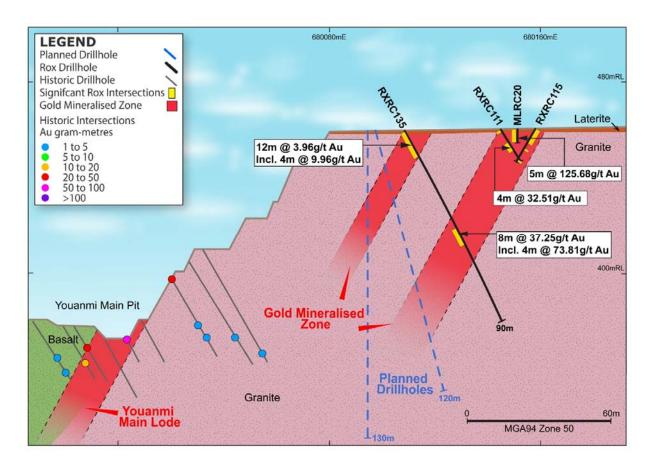
Figure 2 – Cross Section through Main Pit and Grace Prospect showing depth extension and new HW mineralisation
