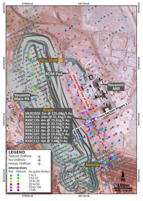
Figure 1 – Aerial photo with drill collars and intersections overlayed
