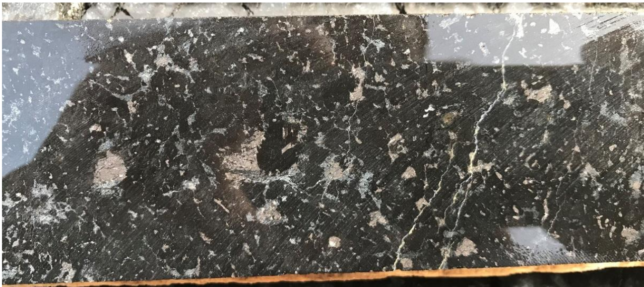
Figure 5: Strongly mineralised disseminated sulfide from 107.3m downhole, drillhole BP20-03 within the King Cobra discovery zone
