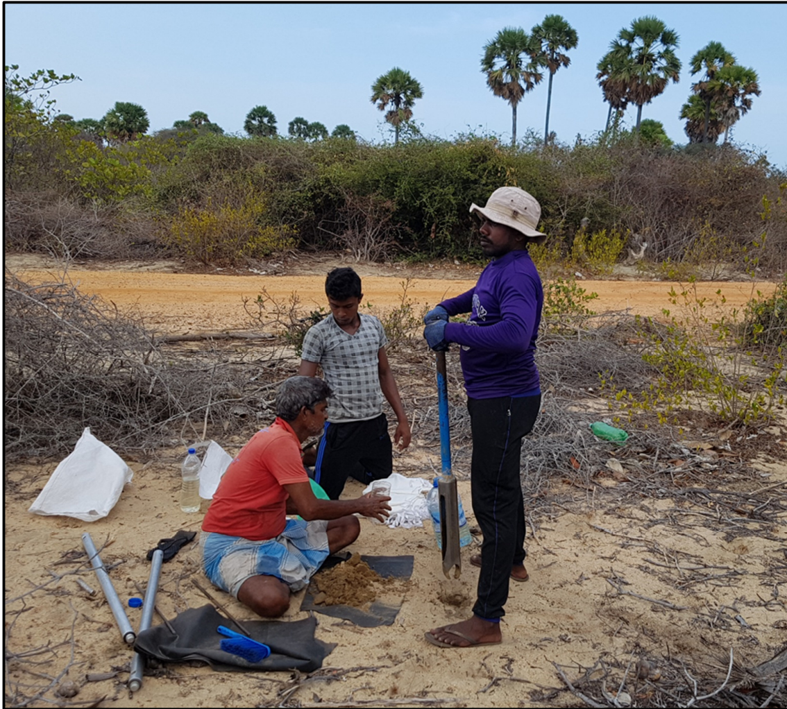
Figure 15 Hand-held auger drilling – twin-hole programme 2018
