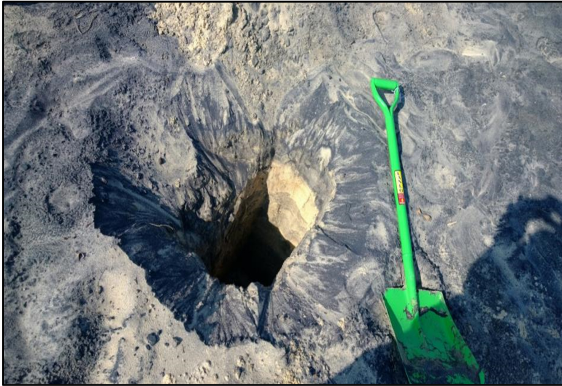
Figure 8 Pit dug into HM mineralisation within berm area (from Badenhorst, 2014)
