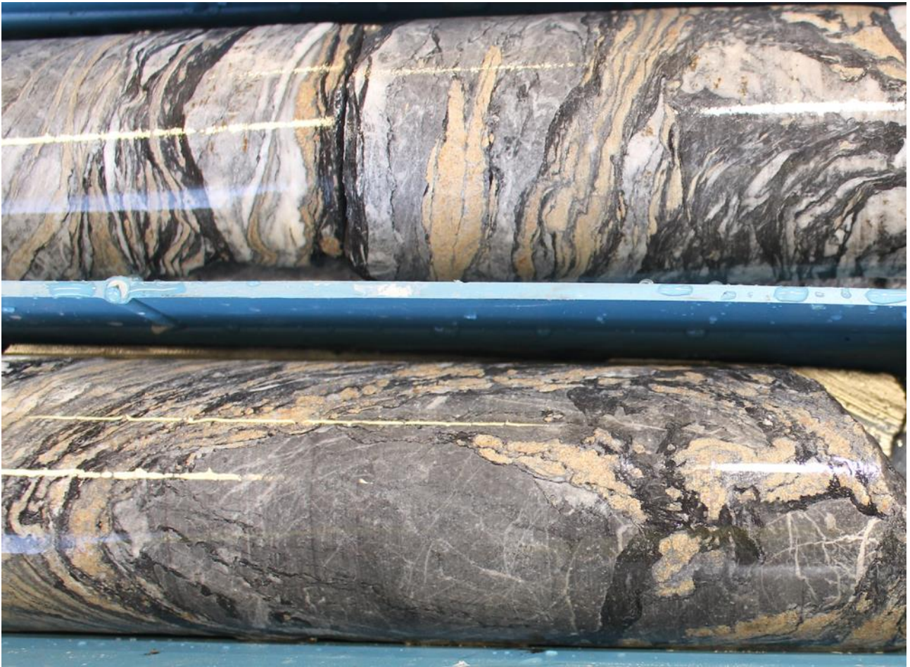
Figure 3: Drill core showing Pian Bracca style mineralisation as honey-coloured stringer sphalerite (from drill-hole PBD02)
