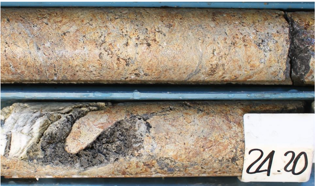
Figure 4: Drill core showing Breno style mineralisation as honey-coloured massive sphalerite (from drill-hole PBD02)
