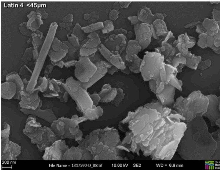
Figure 2: SEMs of <45 micron fractions showing halloysite tubes and kaolinite plates from location 4
