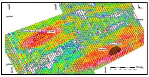
Figure 3: Image of stacked airborne EM CDI sections showing the conductive A4 Dome in proximity to the T3 Dome and the planned T3 Project open pit.
