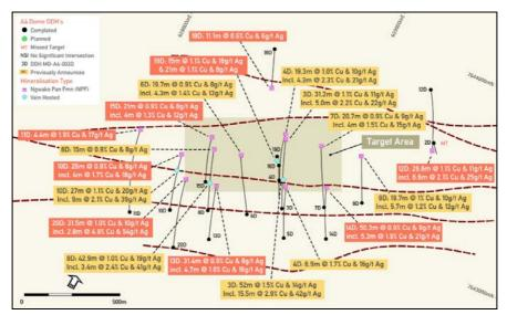
Figure 4: Plan of the A4 Dome Target Area showing significant intersections in previous drilling on 200m spaced sections, as reported by MOD in 2018.
