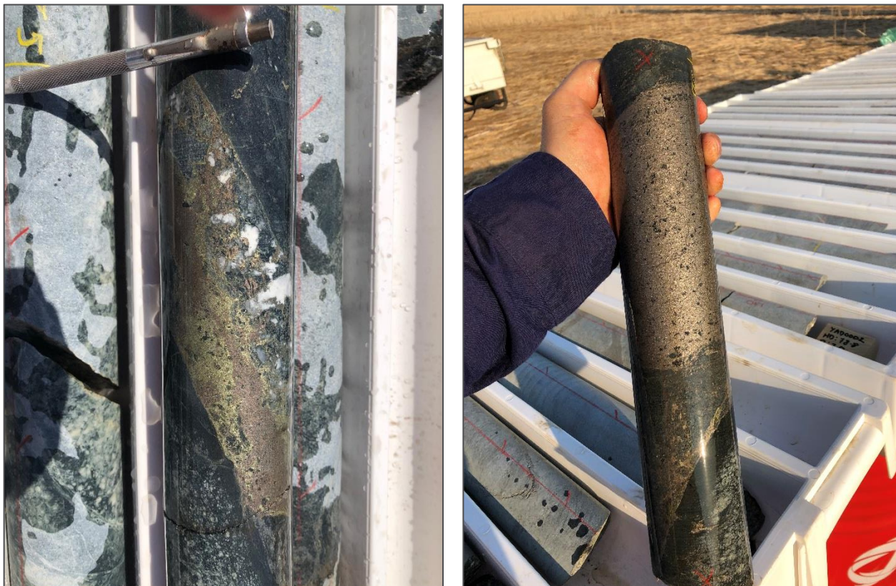
Figure 8. Left: Chalcopyrite and pyrrhotite mineralisation in YAD0001. Right: Massive pyrrhotite mineralisation with minor pentlandite in drill hole YAD0002.
