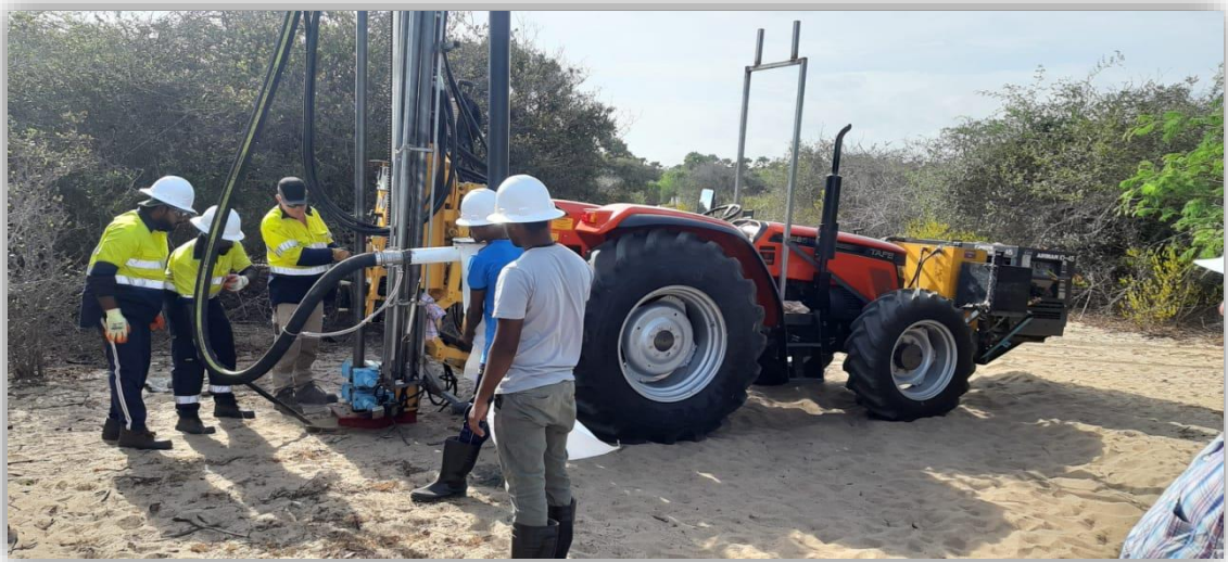
Figure 13 RC aircore tractor mounted drilling rig owned and operated by Titanium Sands Ltd.
