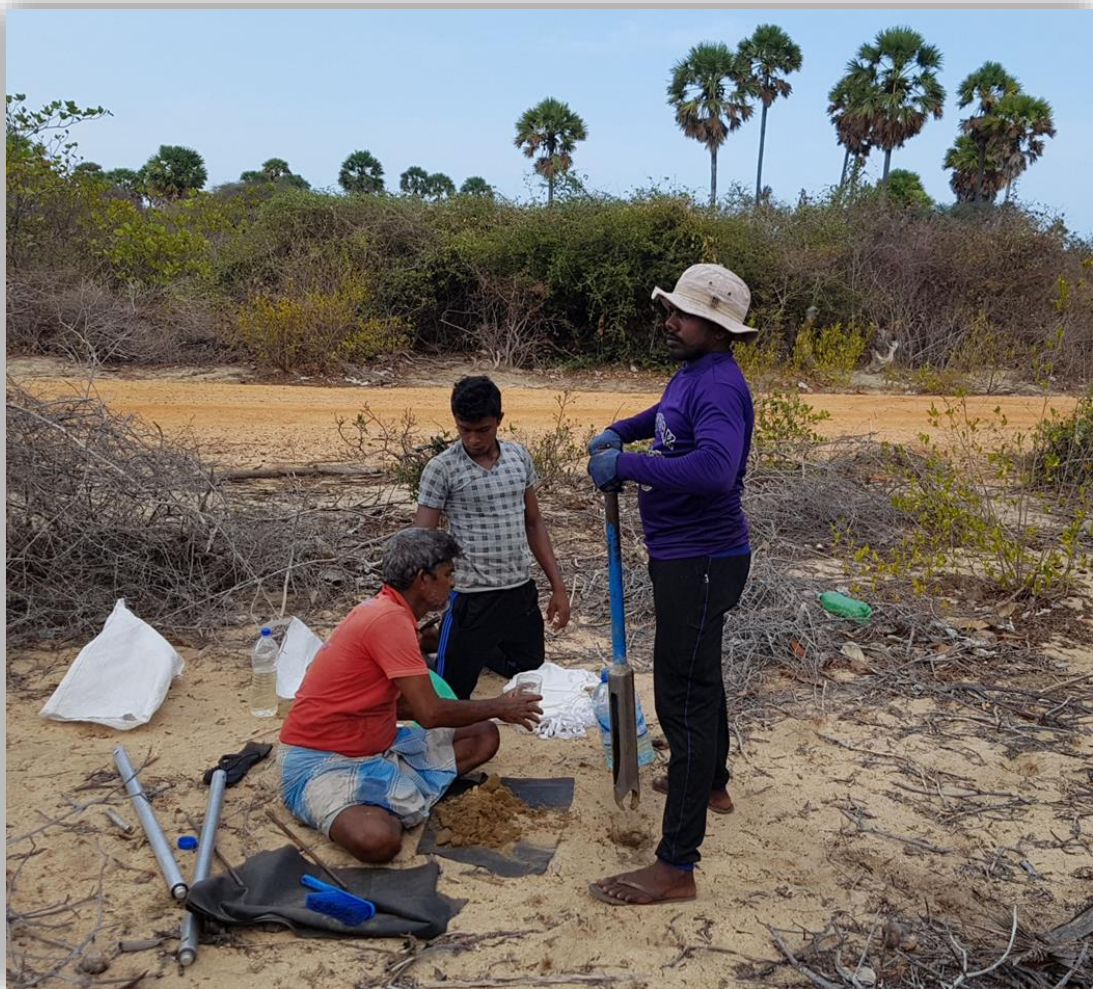
Figure 6 twin hole drilling under supervision by GeoActiv (Pty) Ltd.
