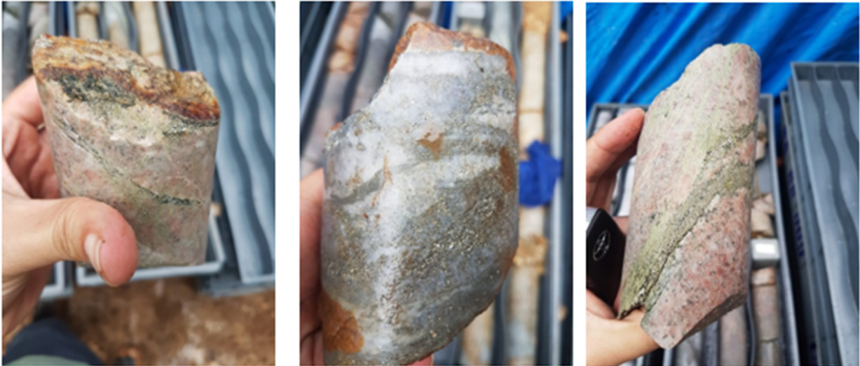
Figure 6: NADD008 - Graça Prospect. Strong pyrite alteration associated with shearing and veins observed down the hole.
