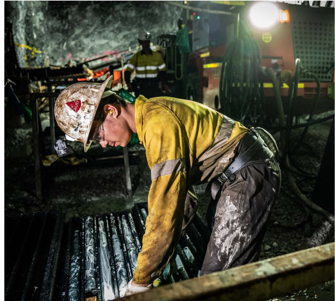
KOTH underground diamond drilling. Driller's off-sider cleaning drill core.
