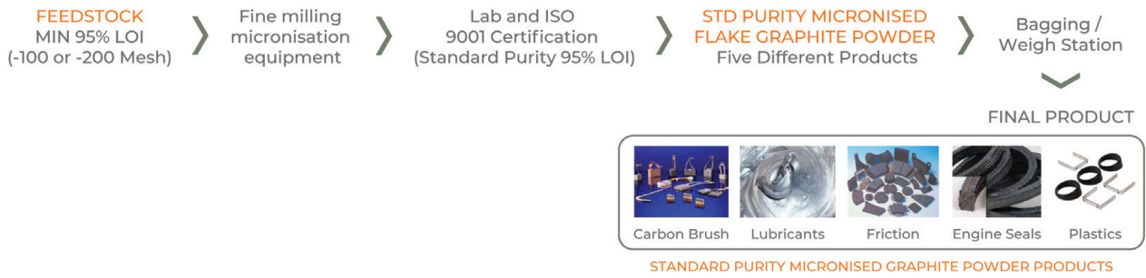
Figure 13: Process flow chart for micronised graphite
