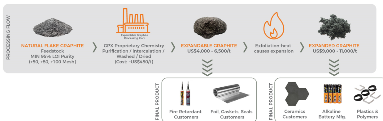
Figure 12: Process flow chart for expandable graphite and expanded graphite
