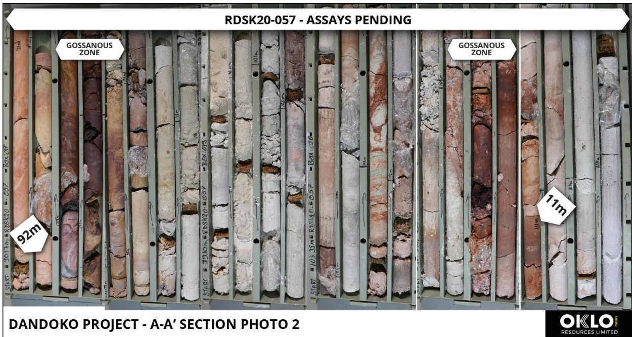
Figure 6: Photo of diamond core from hole RDSK20-057 (92m–111m) showing altered sediments hosting gossanous zones, assays pending
