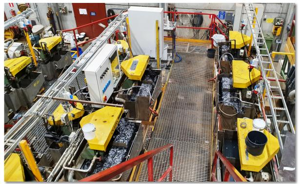
Figure 1 Partial overview of milled Talga graphite ore undergoing flotation concentration stages.
