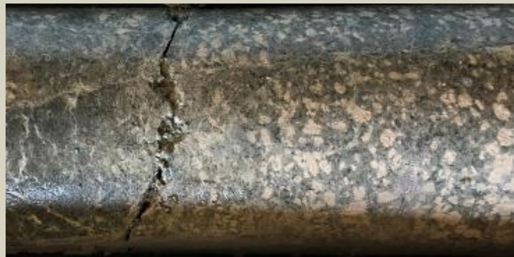
Dacite porphyry, strong pervasive clay+chlorite, complete replacement of feldspar phenocrysts by clay. 59.35m
