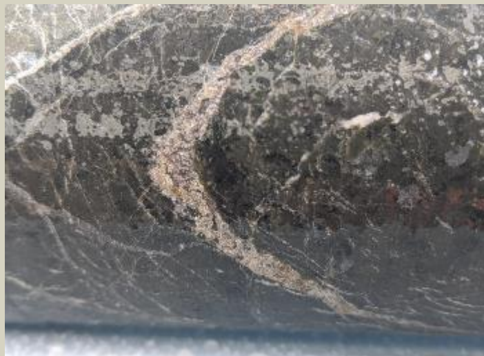
Anhydrite pyrite chalcopyrite vein at 118.8m.
