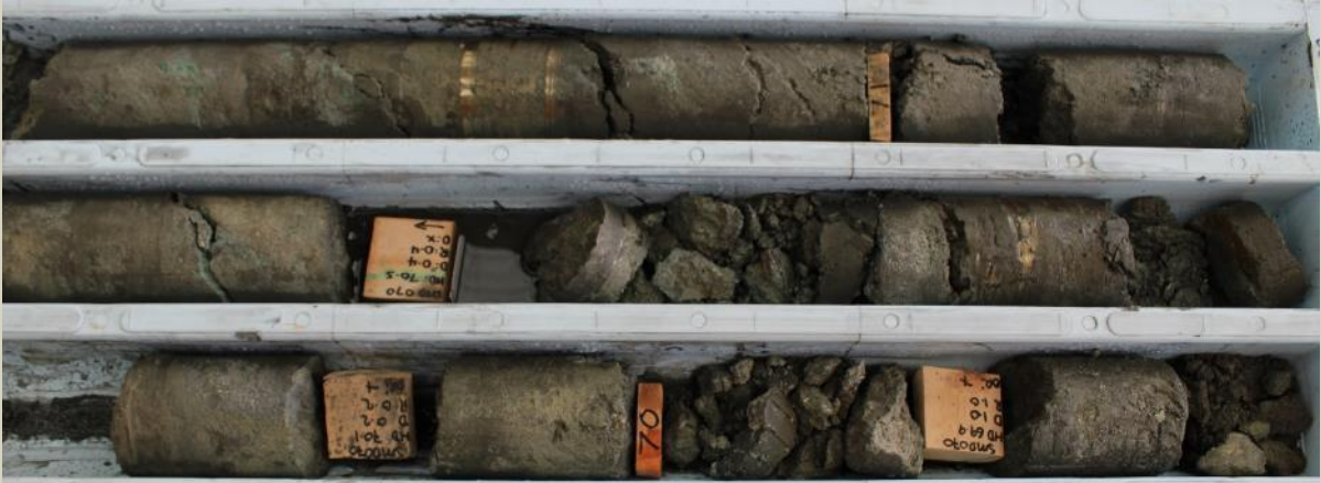
Massive sulphide veining at 70-71m.
