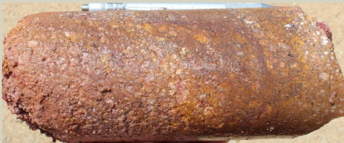
Weathered dacite at 7.8m
