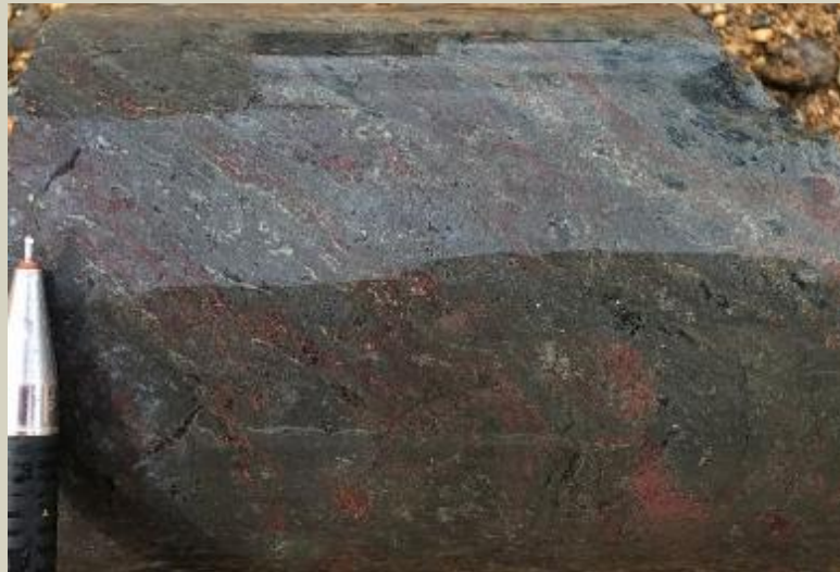
Banded massive sulphide, mostly pyrite with minor chalcopyrite and hematite. 29.7m
