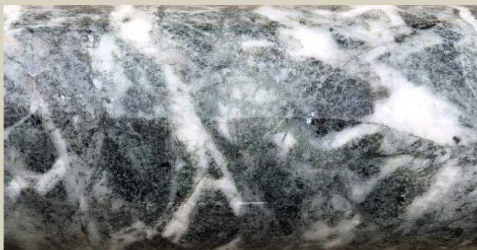
Fragmented quartz+carbonate veins in chlorite+quartz-altered ultramafic. 157.1m
