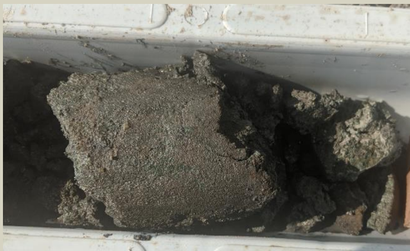
Friable sulphide zone. Dominantly pyrite with fuchsite alteration. At 64.3m.
