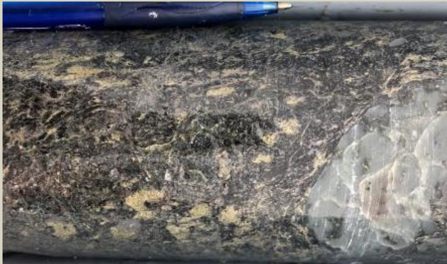
Coarse grained blebby chalcopyrite, together with galena and sphalerite in a coarse sandy unit within the serpentinite. 108.1m
