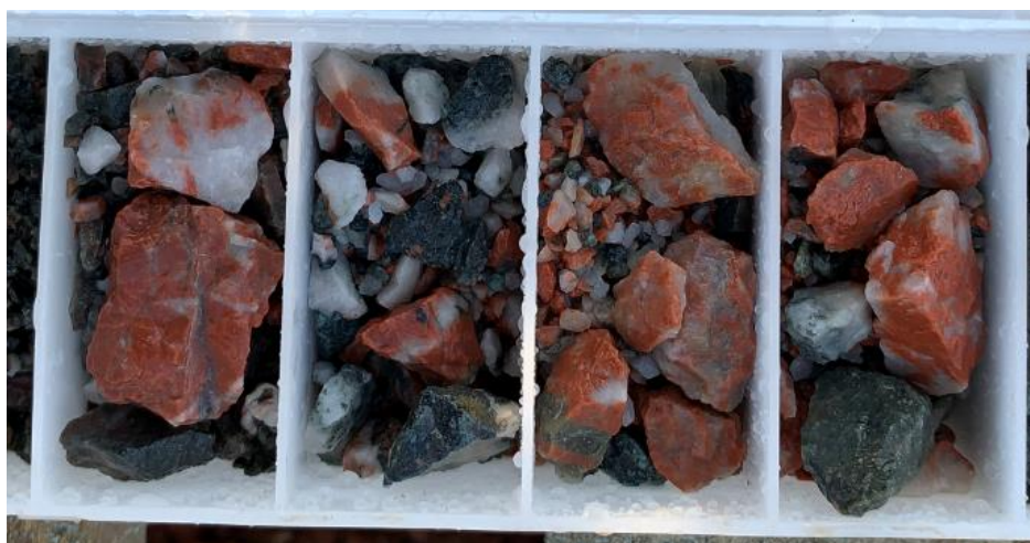
Figure 5 Quartz Adularia Veining from RC drilling at the Central Dome area (KMRC227: 26-30m)
