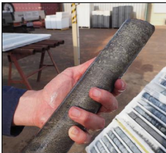
Photo 2 – 3: Massive pyrrhotite – pentlandite (nickel sulphide) – pyrite – chalcopyrite in drill-hole SNDD005 at Saint Patricks: 1.77m @ 6.72% Ni, 0.27% Cu and 0.13% Co from 227.31m down-hole.
