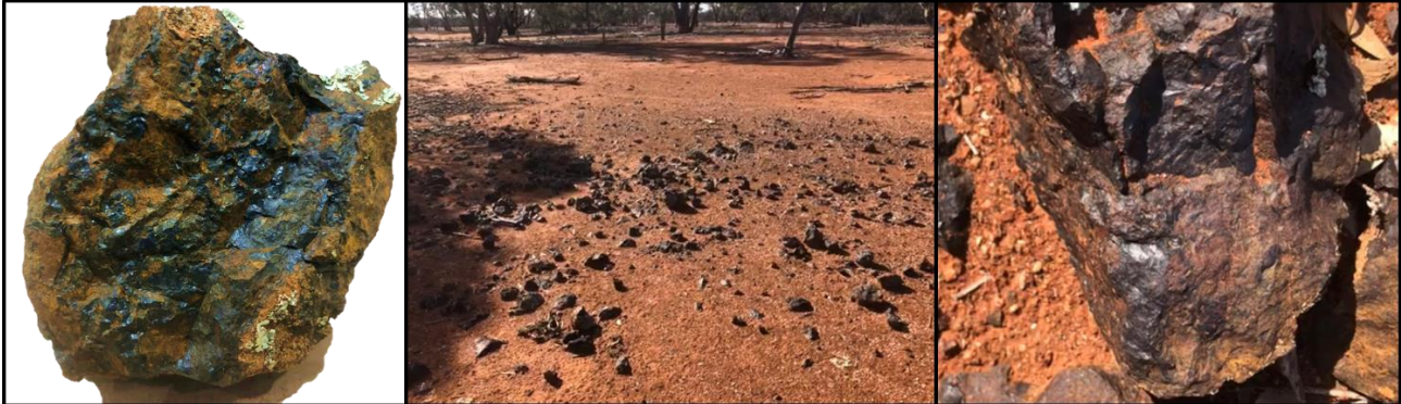
Figure 5: photos of gossan from locations flanking a subtle ridge line running NW, within the Rochford copper in soil anomaly.
