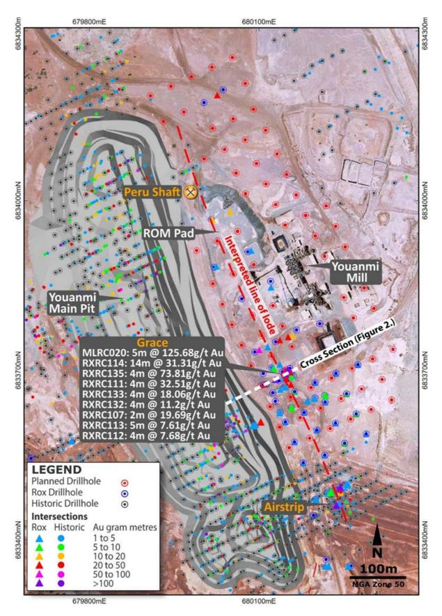
Figure 3 - Aerial photo with drill collars & intersections overlaid
