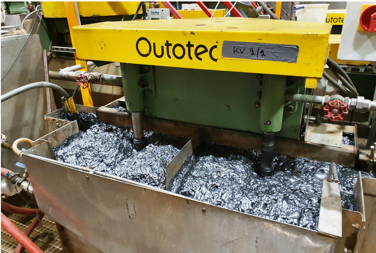
Figure 4. Flotation concentrate of Vittangi graphite ore during 60 tonne pilot process program.
