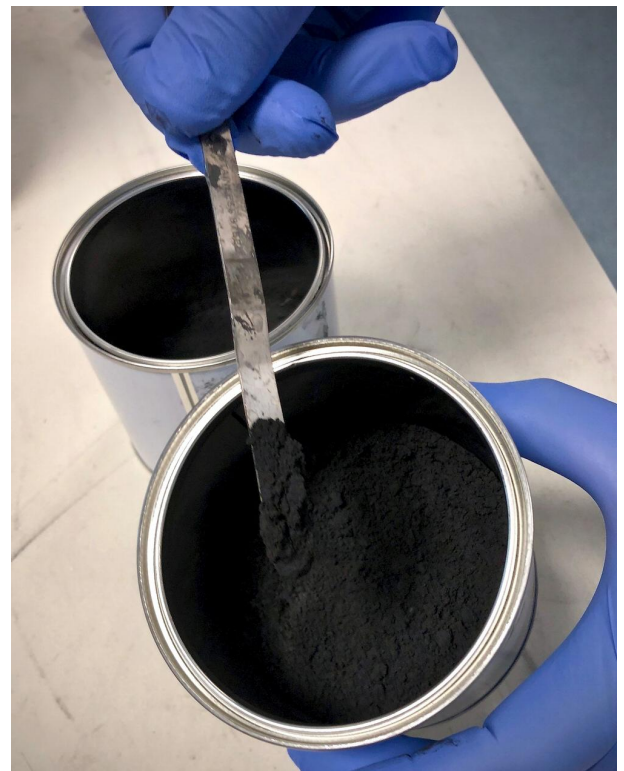
Figure 2. Talga's Lithium-ion battery anode product Talnode®-C during processing.
