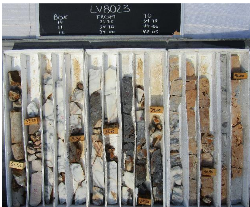
Figure 3: Core from LV8023 showing mineralised interval 34.30 to 39.40 metres of the ore zone.
