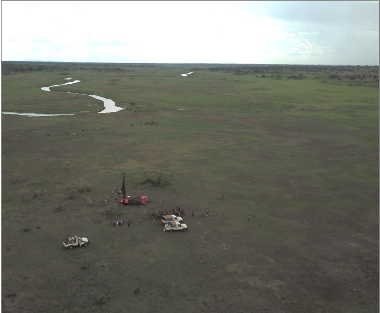
Figure 6. Drone photograph of aircore drilling at Bua Channel. Rutile mineralisation occurs in sand in this wide, meandering channel. The current-day river is approximately 20m wide.
