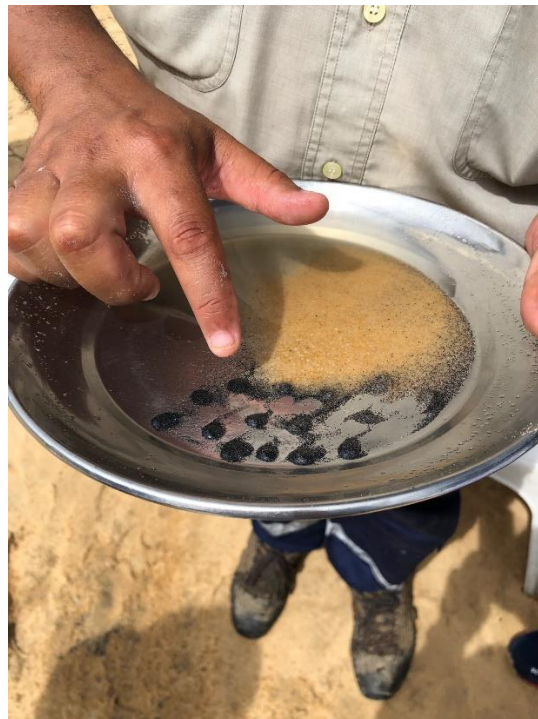
Figure 4 Panning of RC aircore samples from below the water table, during logging at the Mannar Island Project. Dark material is heavy minerals.
