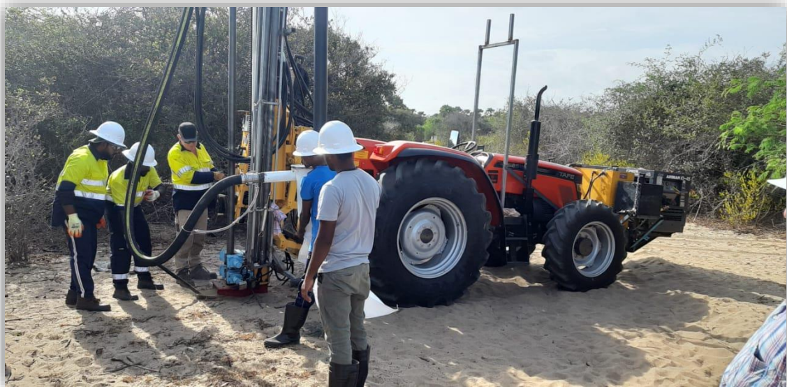
Figure 8 RC aircore tractor mounted drilling rig owned and operated by Titanium Sands Ltd.
