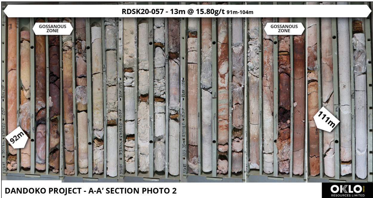
Figure 5: Photo of diamond core from hole RDSK20-057 (92m–111m) showing altered sediments hosting gossanous zones.
