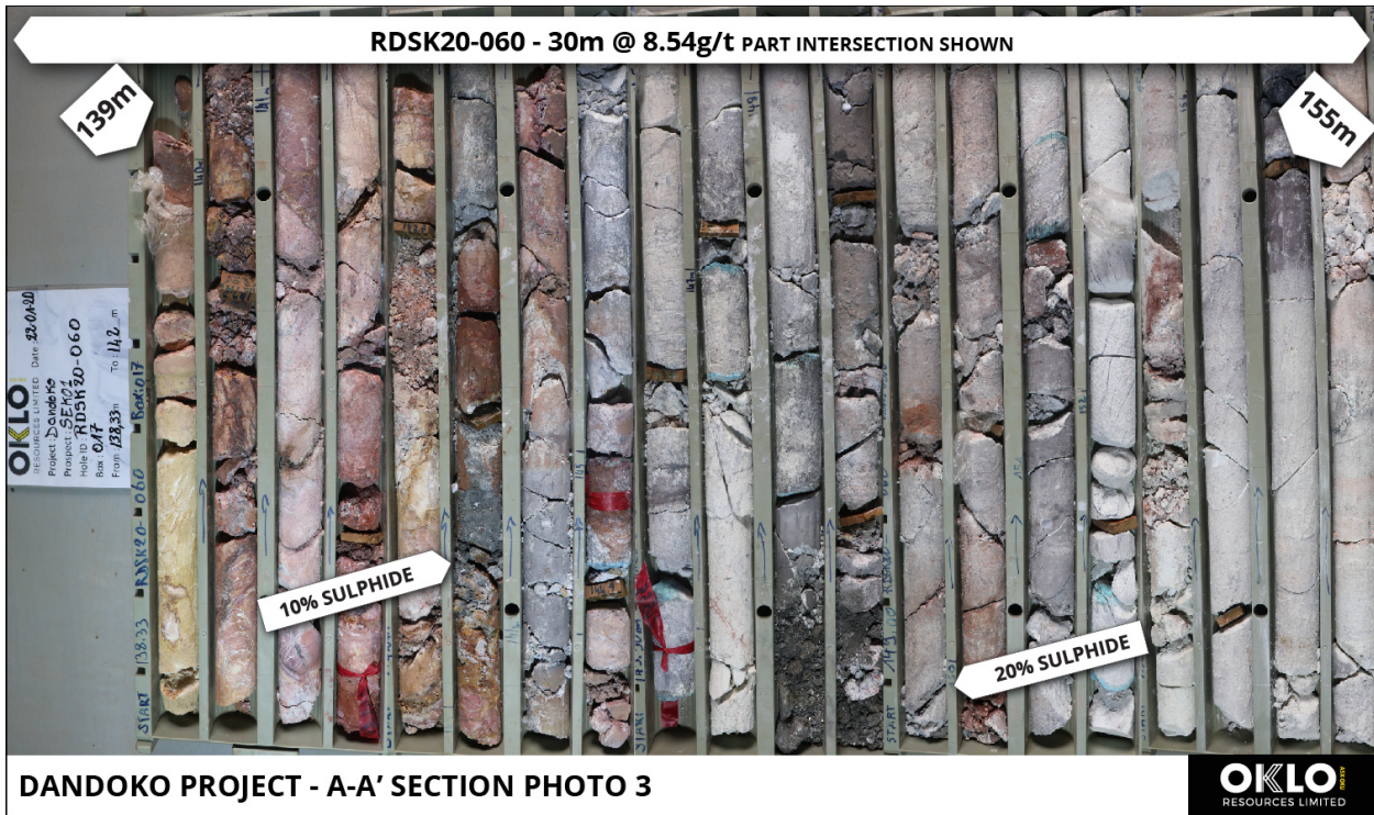
Figure 6: Photo of diamond core from hole RDSK20-060 (139m – 155m), showing altered sediments hosting gossanous and sulphidic zones.
