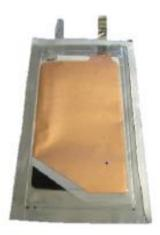
Image 1: Image of a single-layer pouch test cell
