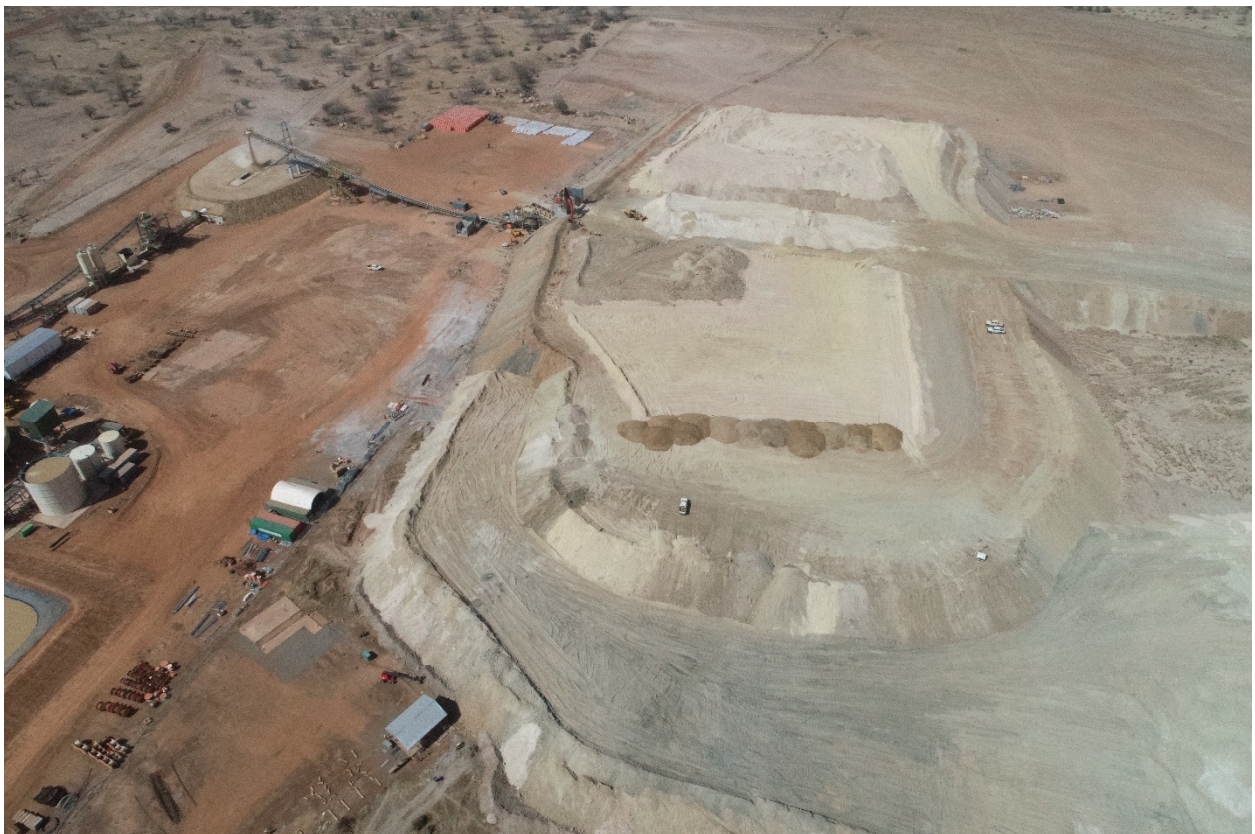
Photo 2: ROM pad stockpiles, primary crusher and coarse ore stockpile
