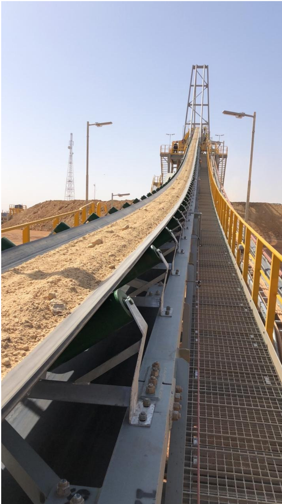
Photo 3: Crushed ore conveyed to the coarse stockpile
