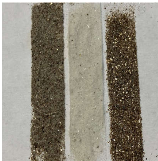
Picture showing the gold plant leach residue (left), non magnetic reject (centre) and mica rich magnetic concentrate (right)
