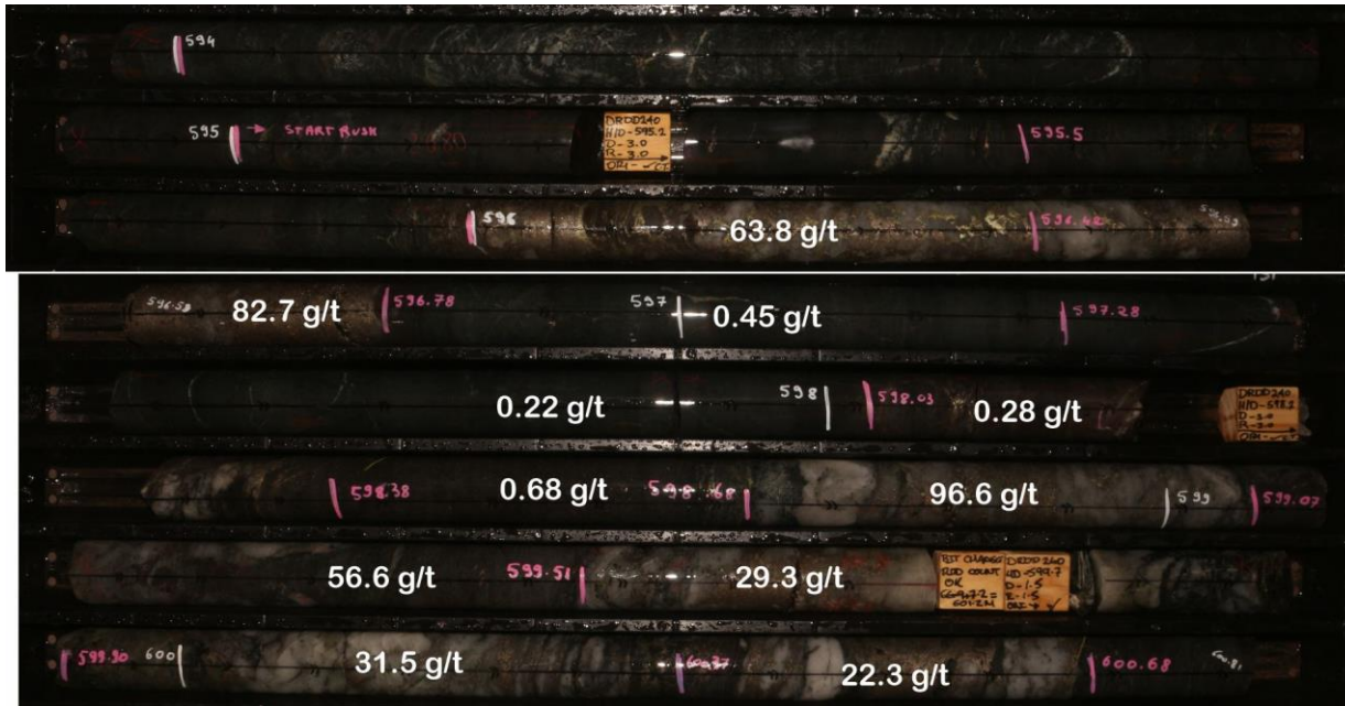
Figure 5: Viago Lode DRDD236. Mineralisation associated with strong biotite altered shearing with sharp strain gradients in hanging wall and footwall to undeformed dolerite. 80% of interval smokey quartz vein hosting 20% sulphide, locally semi-massive (over 40 cm), with typical cataclastic/fracture fill textures. Biotite altered shear observed as laminations within the vein as well as clasts within the sulphide.
