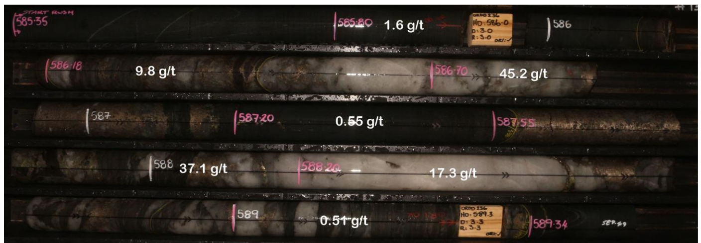
Figure 2: Tribune Lode DRDD360 dominant milky quartz, hosted in moderate biotite/amphibole shearing. Overall 30% sulphide, locally semi-massive with fracture fill to cataclastic textures, chalcopyrite minor with pyrrhotite dominant. Interval assayed 3.2 m @ 9.8 g/t gold.
