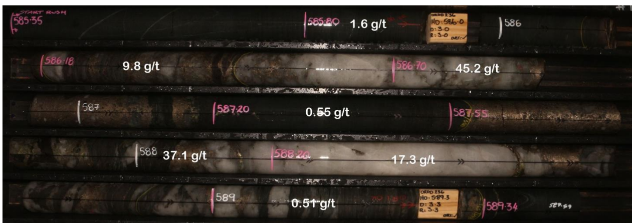
Figure 5: Viago Lode DRDD236. Mineralisation associated with strong biotite altered shearing with sharp strain gradients in hanging wall and footwall to undeformed dolerite. 80% of interval smokey quartz vein hosting 20% sulphide, locally semi-massive (over 40 cm), with typical cataclastic/fracture fill textures. Biotite altered shear observed as laminations within the vein as well as clasts within the sulphide.
