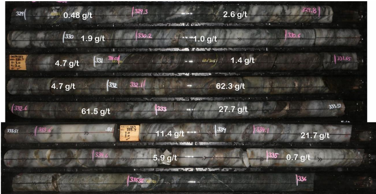
Figure 1: Tribune Lode DRDD337 mix of smokey and milky quartz, hosted in moderate biotite/amphibole shearing. Overall 20% sulphide, locally semi-massive with fracture fill to cataclastic textures, chalcopyrite minor with pyrrhotite dominant. Overall +40 flecks of visible gold. Interval assayed 5.7 m @ 17.4 g/t gold
