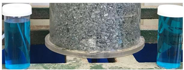
Image 1 / Metallurgical column test-work
