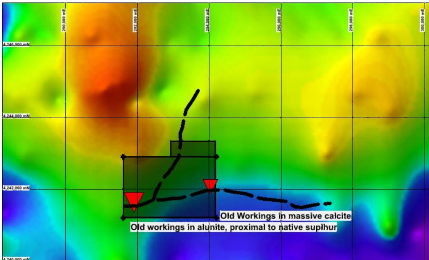
The image above shows the main structural elements at White Mountain (thick black dashed line), on top of the regional aeromagnetics (reduced of the pole, first vertical derivative). Old workings
