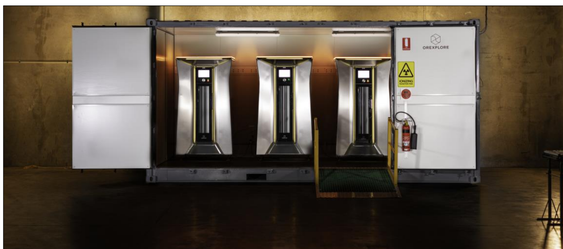
Fig 2. Orexlore field container with three GeoCore X10 instruments capable of scanning over 5,000m of core per month generating unique 3D tomographic imaging, through the core geochemistry and a host of other automated outputs.
