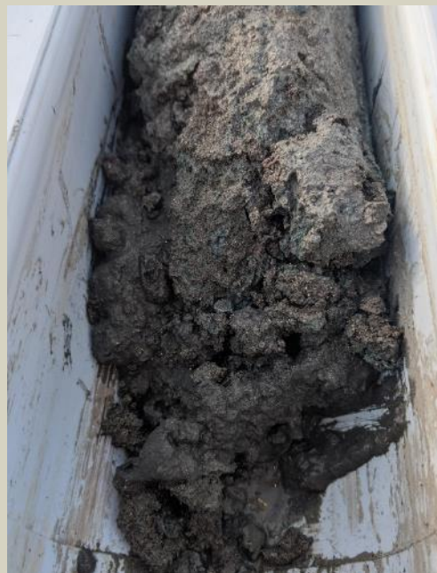
Sulphide clay zone at 183m.
