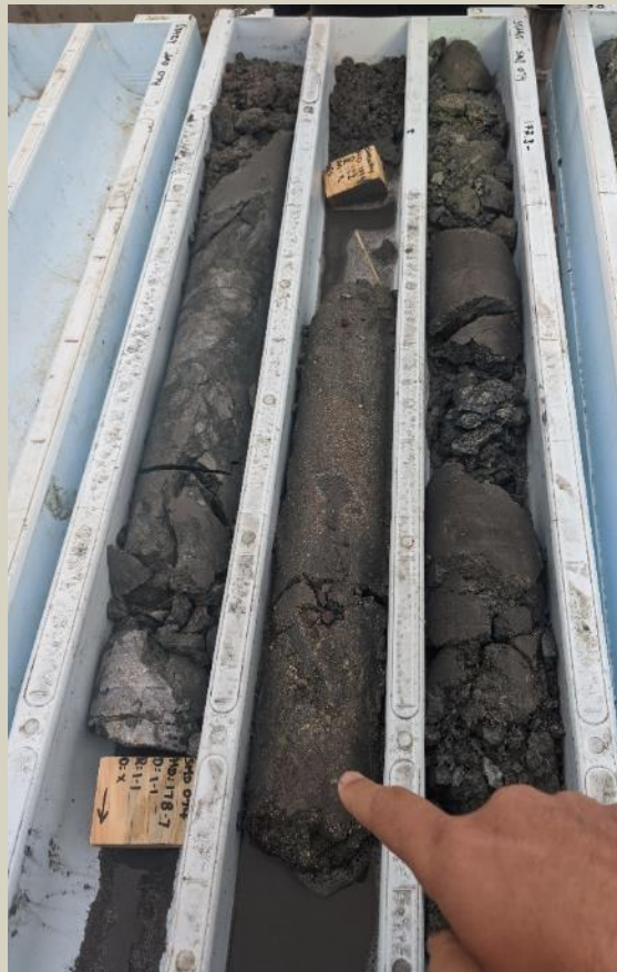
Friable pyrite and chalcopryite zone in the UCF at 178m.
