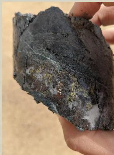
Quartz hematite chalcopyrite vein at 153.2m
