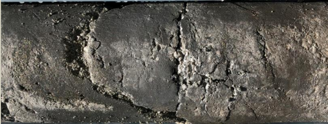
Pyrite+chalcocite vein with sericite halo. 33.6m
