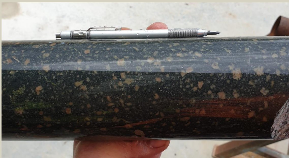
Dacite with hematite dusted feldspar phenocrysts and disseminated pyrite at 272m.
