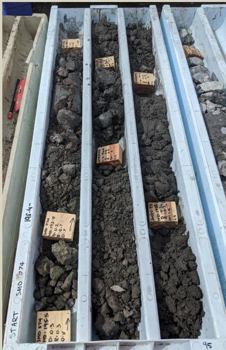
Massive sulphide veining in UCF at 195.5-197.6m.
