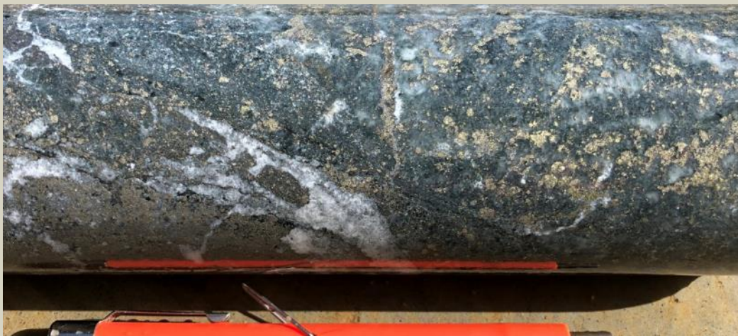
Contact between massive pyrite+sphalerite zone with quartz+dolomite-altered serpentinite with disseminated and patchy pyrite, sphalerite and chalcopyrite. 361.4m
