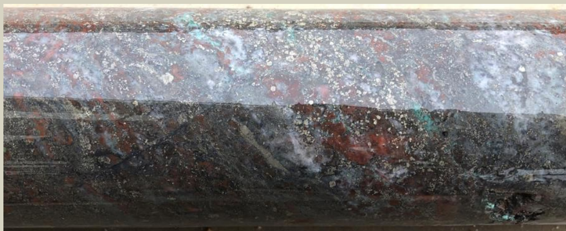
Pyrite in strongly foliated quartz+hematite+fuchsite-altered rock. 230.5m.
