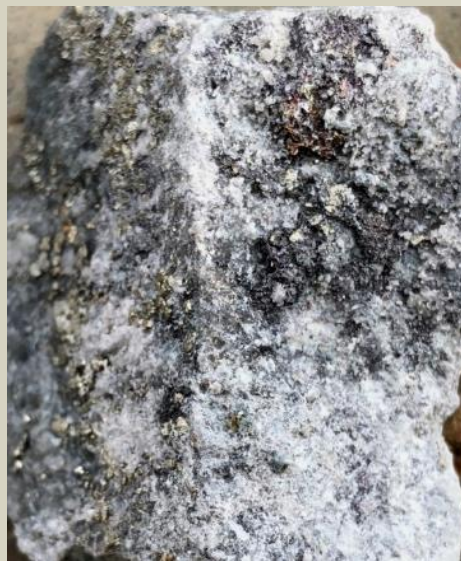
Bornite and chalcocite on fracture. 68.1m
