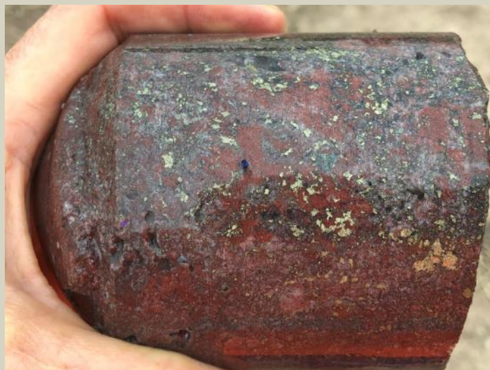
Disseminated chalcopyrite in quartz+hematite rock. 223.4m.
