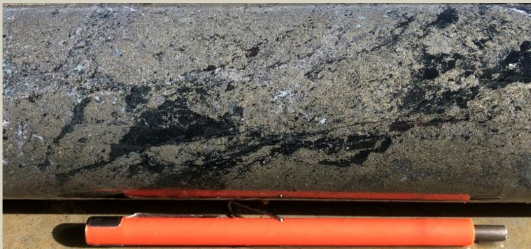
Massive pyrite+low-iron sphalerite. High-grade Zn interval. 361.0m
