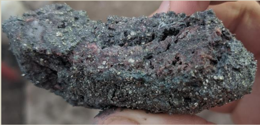
Vuggy quartz, hematite, pyrite and chalcopryite zone in the UCF at 177.4m
