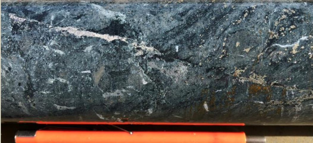
Serpentinite with shear fabric, cut by low-iron sphalerite vein and containing disseminated pyrite.
