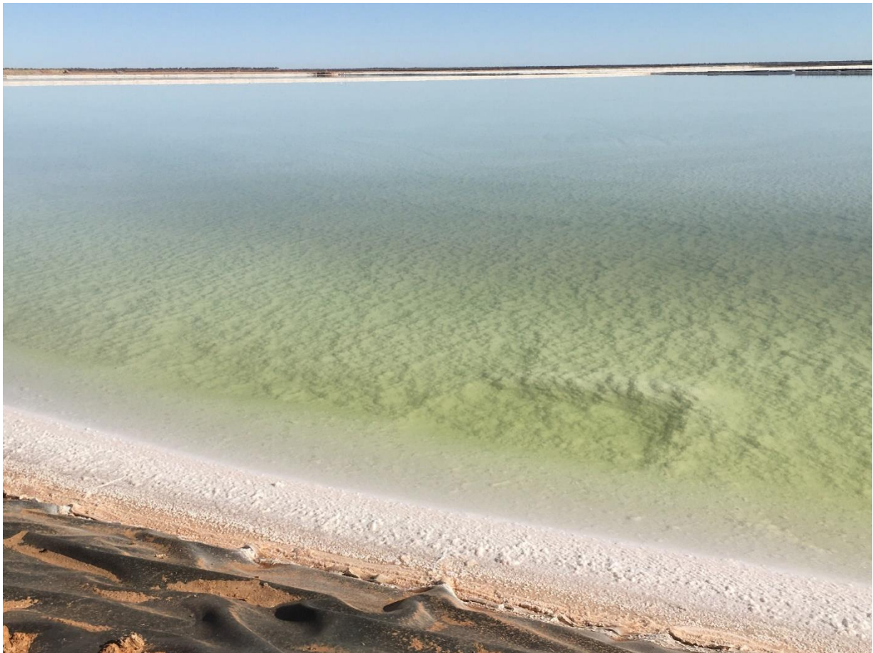
Figure 6: Stage 2 ponds precipitating first salts
