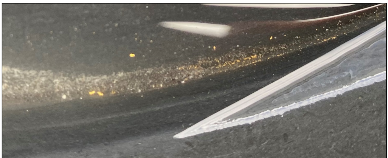
Figure 1 – Panned gold from a small sample of ABFR0273, 38-42 m (4 m at 5.78 g/t gold). View is approximately 20 mm across.
